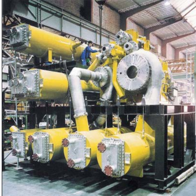
Figure 2 – MAN Turbo 10-stage 200:1 CO 2 Compressor
